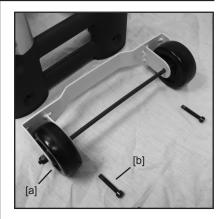
Store the Allen Wrench [a] in the cover of the electrical box. This wrench can be used to adjust the tilt / swivel resistance (see page 6).
